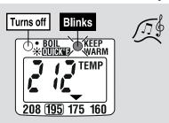
When the boiling process has completed, a melody sounds, the BOIL light turns off, and the KEEP WARM light begins to blink.
