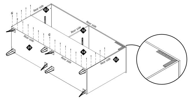
Connect the part 15 onto the part 14, and connect the part 13 into the part 15. And then, connect the part 13 using the hardware (G).
