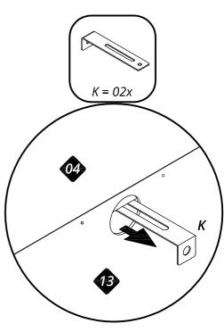
Then, pass the hardware (K) through the hole of the part (13) from inside to the outside as shown in the figure above until it reaches the wall.
