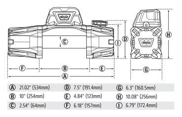
**Winch Dimensions:** 21" L x 6.3" D x 10.1" H (534mm L x 160.5mm D x 256mm H)
