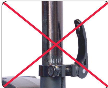
Fig. 4.2 Incorrectly Installed Seat Post
