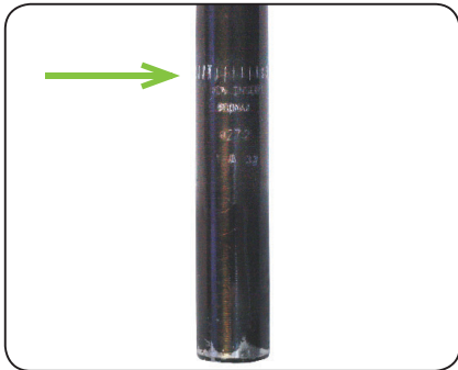
Fig. 4.1 Seat Post, “Minimum Insert Line”
