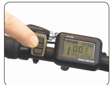
Fig. 10.2 Hold down “MODE” Button for 2 Seconds
