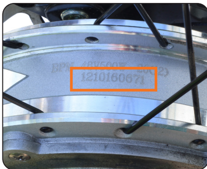
Fig. 13.3 Motor Serial Number Location
