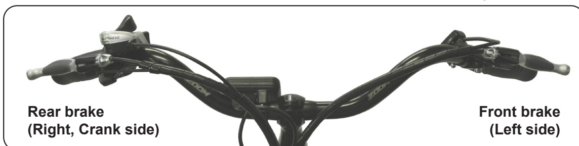
Fig. 1.1 Handlebars (viewed from the front of the bike)
