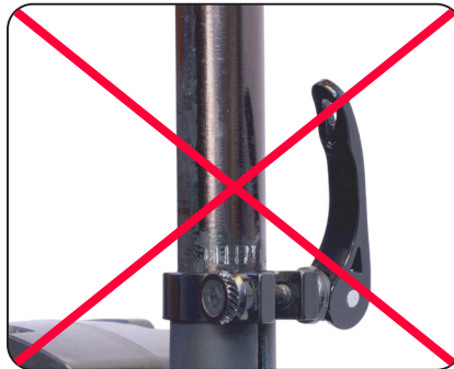
Fig. 4.2 Incorrectly Installed Seat Post
