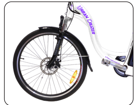
Fig. 2.7 Forks Secured Onto Front Wheel
