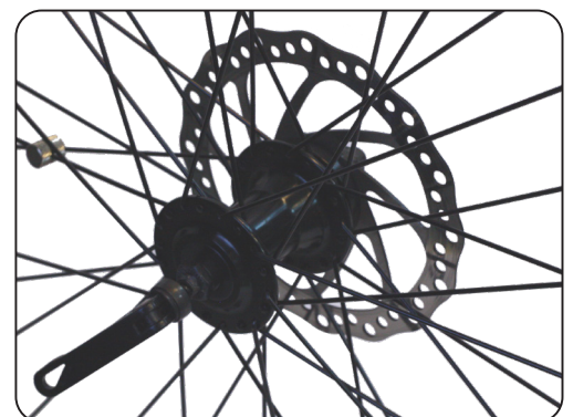
Fig 1.8. Quick Release Lever, Front Wheel
