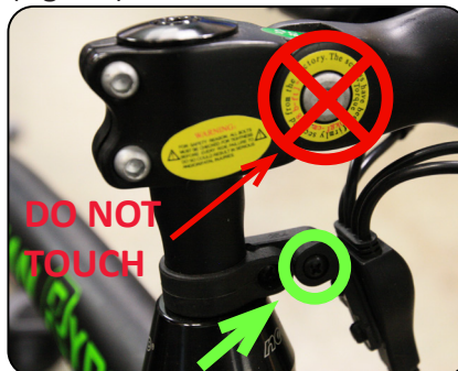
Fig. 1.6 Tighten Cable Screw (green)
