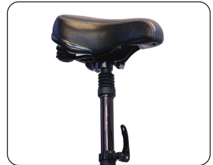
Fig. 4.3 Seat Post Inserted Correctly, 1/4” Past “Minimum Insert Line”
