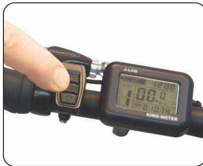
Fig. 9.2 Hold Down “MODE” Button for 2 Seconds
