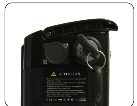
Fig. 8.3 Battery Key - OFF
