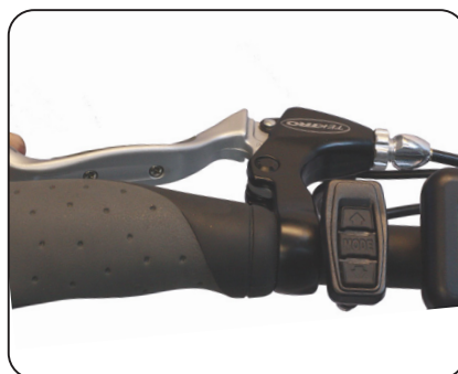
Fig. 8.2 Keep Brake Lever Depressed
