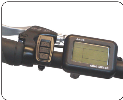
Fig. 9.1 King Meter® Display, OFF
