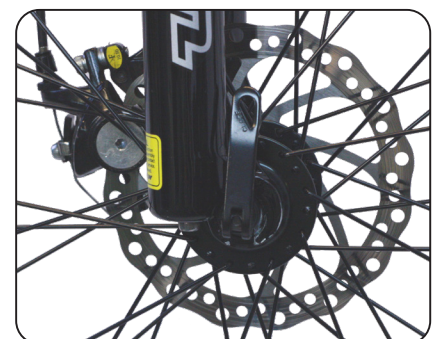
Fig. 2.5 Quick Release Lever In Closed Position
