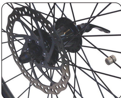
Fig. 2.3 Front Wheel, Quick Release Inserted Into Wheel Axle
