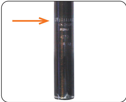
Fig. 4.1 Seat Post, “Minimum Insert Line”
