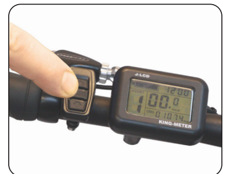
Fig. 10.2 Hold down “MODE” Button for 2 Seconds
