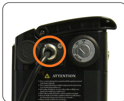
Fig. 7.2 Battery Charging Port
