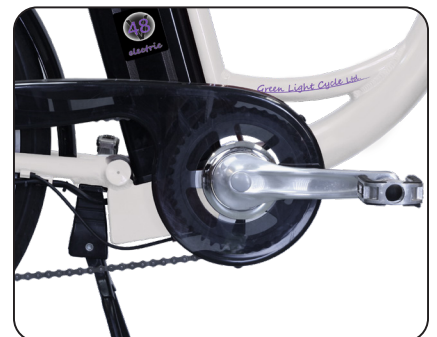
Fig. 3.2 Crank Arm, Right Pedal Inserted
