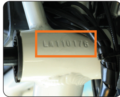
Fig. 13.2 Frame Serial Number Location
