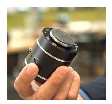
The Soundwaver is a battery-powered Bluetooth receiver with a sound pressure transducer. It transforms any hard surface such as wood, glass or metal into a speaker which you can use to listen to your music in stunning sound quality. Various devices such as computers, laptops, tablets or smartphones can be connected via a 3.5 mm audio connector or via Bluetooth V2.0. The Soundwaver can be recharged via a USB port, for example on a computer.
