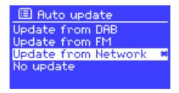
Network uses a time signal sent from the Frontier Silicon Internet radio portal when in any network connected mode.
