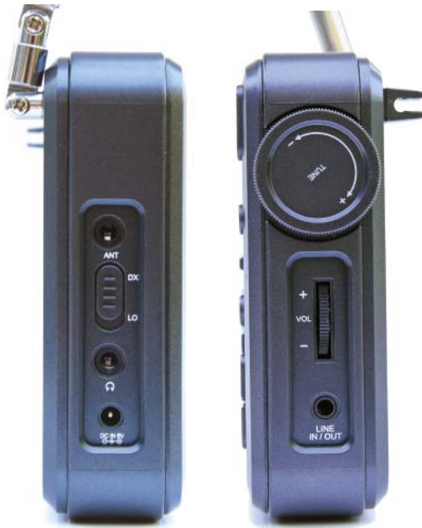
Figure 3 — The left side of the receiver has an external antenna jack, a DX/local switch to reduce gain if the receiver overloads, a stereo headphone jack, and an external power jack. The right side includes tuning and volume controls and a line in/out jack.
