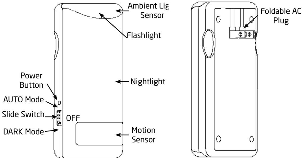
**Power Button** - Turns the device on manually. After plugging the Blackout Buddy Connect Color into AC power press and release the Power Button and the Nightlight will start cycling through the available colors. When the desired color appears on the Nightlight press and release the Power Button again to lock in that color. Leave the BB Connect Color alone and it will automatically operate per the Mode chosen with the Slide Switch.
