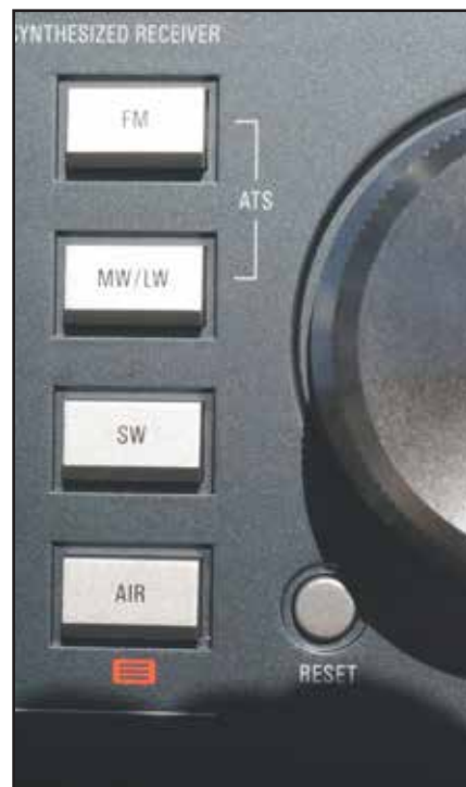
Mode buttons make changing bands easy. Push the MW / LW button twice to get to the low-frequency beacon band.
