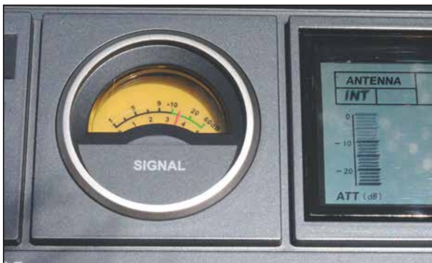
The analog S meter allows you to see incoming signal strengths, and watch HF shortwave peaks and valleys of reception, due to ionospheric conditions that are always changing.
