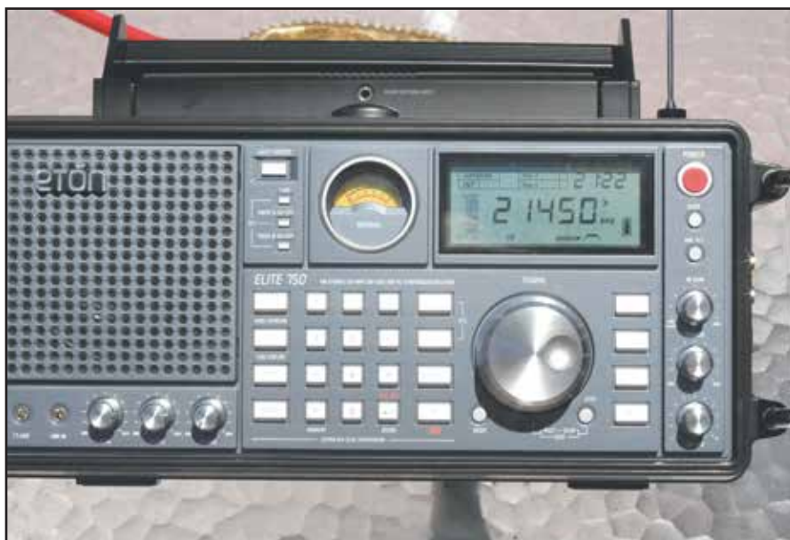
The large LCD display makes tuning in frequencies a snap. Here we are tuned in to 15 meters, ham SSB reception, using the BFO to tune in upper sideband, or lower sideband on lower ham bands, plus CW and data.
