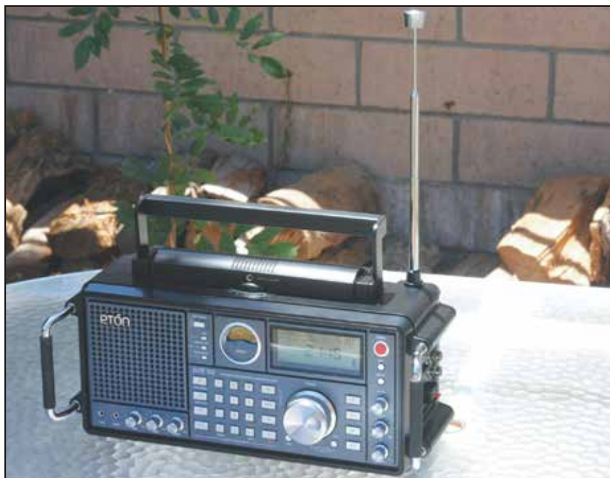
This large-sized Eton 750 portable receiver boasts full-fidelity AM radio reception, air band, and stereo FM reception, in addition to the low frequency beacon band and ALL shortwave bands from 1.7-30 MHz non-stop, AM or SSB.
