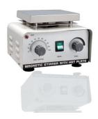
**Specification**: It has a compact stirring device utilizing a rotating magnetic field (created by a PERMANENT MAGNET) which induces variable speed stirring action. Stirring is accomplished by means of small tefflon rotor, which when placed in the liquid to be stirred is capable of rotation by magnetic field applied from below the container. The unit is fitted with pilot lamp
