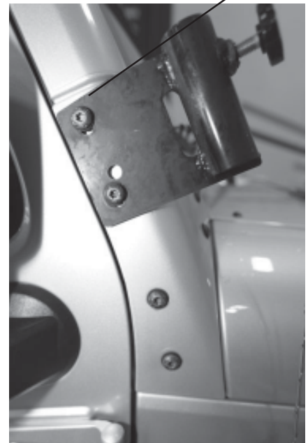
Figure 1.1 Bracket Mounting Location On JK
