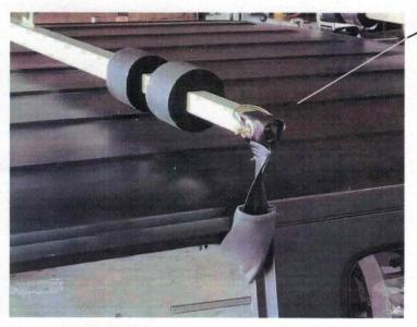
Slide the looped end of each Straps on the end of the Bridge and align the holes in the strap with the hole in the Bridge. Pin the straps to the Bridge through these holes with the Safety Pins.
