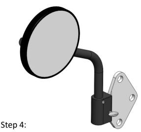
Tighten the mirror block to the door hinge with the provided thumb screw. Move and adjust the mirror head to the desired position and then tighten with the provided set screw and hex key.
