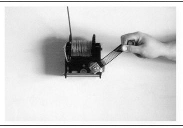
With the cable coming straight up out of the frame as shown, reattach the spool. Then attach the supplied turning handle.
