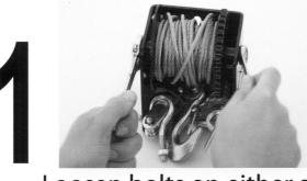
Loosen bolts on either side of hand crank unit
