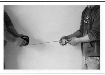
With a helper unwind the cable from the spool. This is done to reverse the direction of the cable as shown in step 8.
