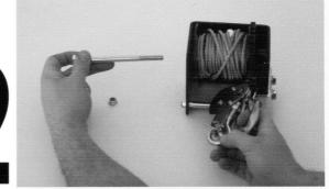
Remove bolt and set spool of wire-cable aside.
