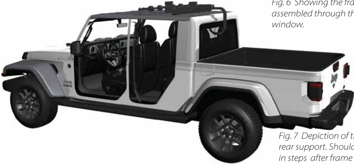
Fig.2 Front Assembly placed on Jeep before clipping in the rear assembly
