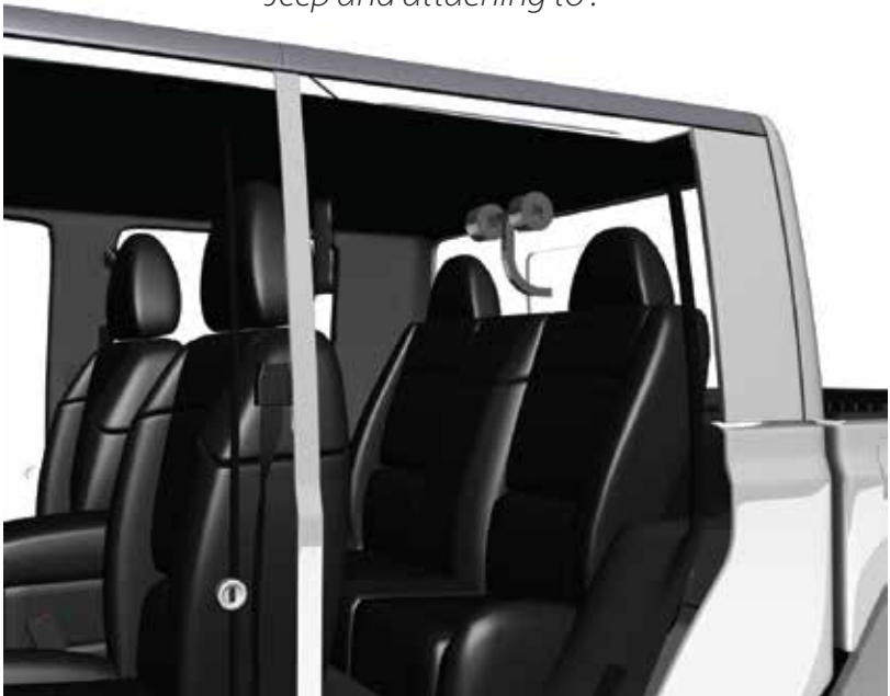
Fig. 5 Placing the support arm through the rear window of the Jeep and attaching to .
