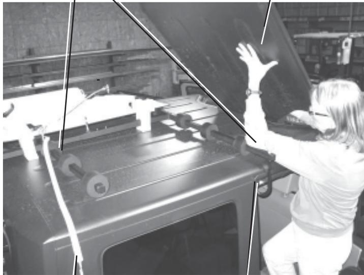
Move the bungee cord to the back as shown to avoid getting in the way of the top section being placed on the hoist frame.
