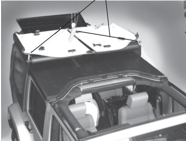
Slide top section into the foam stand offs and center top section. Stretch cord over top section on the diagonal and hook to front eye bolt.
