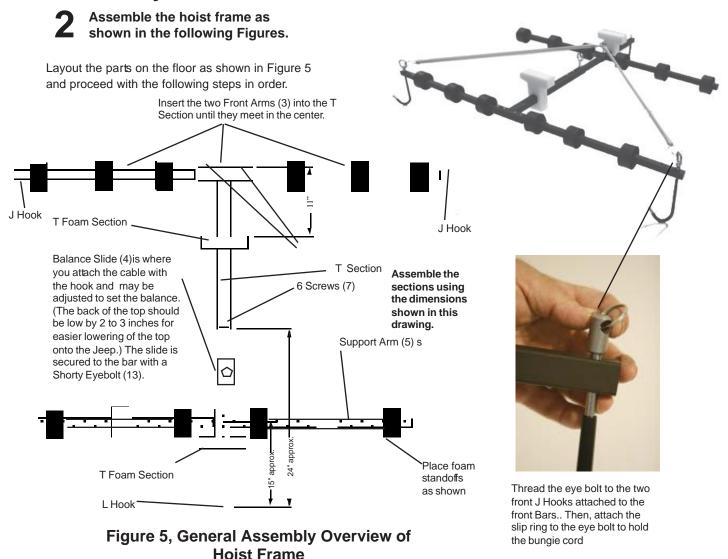
Slide Foam Protectors (12) on each of the Frame Arms (3) and on the Top Section Support Arms (5) as shown in Figure 5. Use soapy water to ease the installation of these foam parts and orient each as shown in Figure 5.
