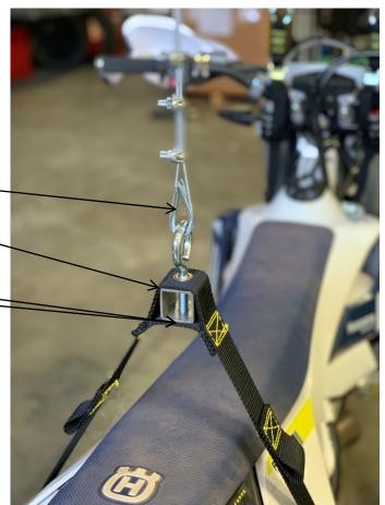
Loop the bottom of the strap around your swing arm on each side. Avoid trapping any cables.
