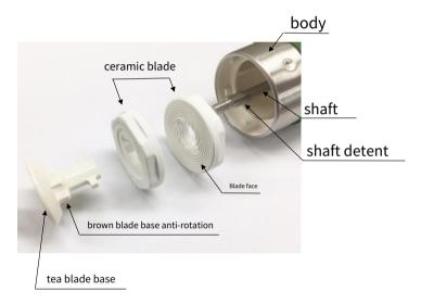
①Align the blade whirl-stop on the outer circumference of the blade with the body whirl-stop inside the body.
