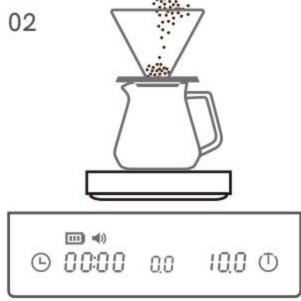
Put a brewer on the platform and saturate the paper filter. Turn it on and quick press to tare. Put ground coffee with desired weight into the filter. Quick press the Tare button again.
