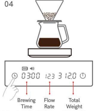
When brewing finishes, quick press the timer button to pause timing and the weighing panel will display your brewing data.
