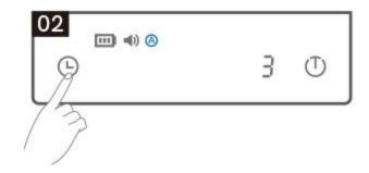
Quick press the timer button 5 times until an audible beep and the Pour-over Auto Timing Mode indicator lights up. Place a brewer on the platform and add ground coffee. Then quick press the timer and wait for a 3-second countdown.
