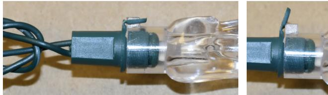
6. With a pair of pliers, grasp the Green 'cap' of the LED. DO NOT grasp or pinch the white, glass portion of the LED element. Gently pull the LED element away from the slot. Please properly dispose as electronic waste.
