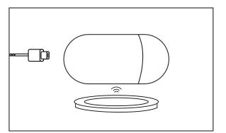
**3.** When placing or removing the earbuds in the capsule, the LED will blink Green.
