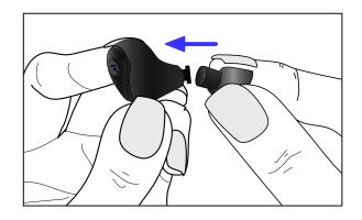
**3** Flip the gel tip back to its original position and ensure it is securely attached before use.
