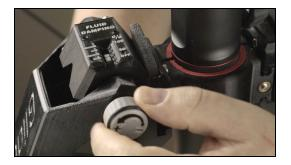
4) Turn both payload adjusters until the gimbal lifts up enough so that it won't bottom out during your test shot. Make sure both sides are evenly angled up or
