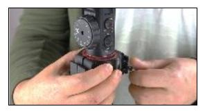
2) Slide mounted gimbal onto Glider and lock down the quick-lock lever so that it sits close to horizontal.
