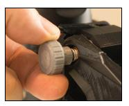
4) Turn the payload adjuster until the gimbal lifts up enough so that it won't bottom out during your test shot. The support
