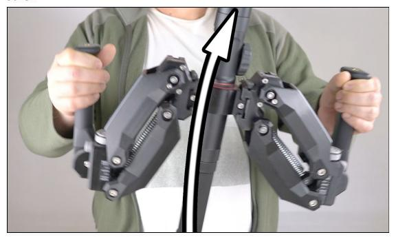
If your gimbal bounces say to the right then the right Payload Spring is weaker than the left and you need to increase the payload adjuster tension on the right side to even it up with the left. When your gimbal bounces straight up you're all set to start your test shot!
