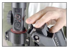
6. Now you finally test the holding power of the gimbal clamp by gripping the gimbal firmly and trying to rotate the 4th axis handle. If the gimbal rotates inside the clamp then tighten the clamp bolts another quarter turn and try again and repeat until it won't move easily.
