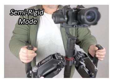
on the handles to lift or lower the gimbal so that the majority of the suspension is mostly locked and you can do your controlled rapid movement. This takes a bit of practice but if you do these transitions like whip pans regularly then it's well worth the practice to get it right.
