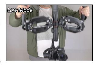
shots. Of all the stabilizer positions this is the easiest mode to operate as the lower centre of gravity keeps the gimbal nice and and smooth with minimal effort.
