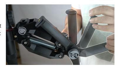
for a narrower grip and more compact form. Once both sides are at the same angle just tighten up the Rosette knobs making sure that the rosette teeth are meshed together and locked in place. You don't need to overtighten these knobs, just tighten until you meet a firm resistance. You may find if you're shooting for instance while 'crabbing' to the side that adjusting the handles independently to different angles may be more ergonomic for you.
