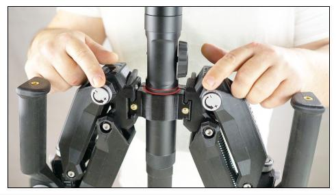
On each side of the gimbal mount are the two smaller adjuster knobs for the variable fluid damping cartridges. The suspension springs, by their nature when stretched bounce back and forth until the springs initial energy or bounce is lost in the system via friction.
