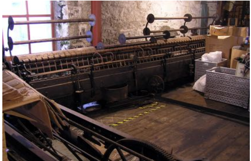
The Platt spinning mule of 1870
