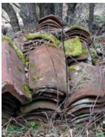
Clay pantiles stored on site
