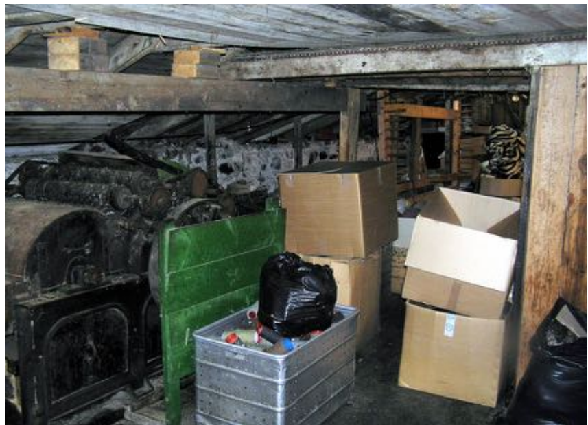
The attic floor – the machine on the left is an early wool blender, or 'teazer'
