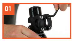
Undo the four face-plate bolts on the front of the stem and remove the face (front) plate.
