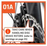
Ensure that the disc rotor is lined up with the gap between the disc pads. When moving on to step 02 (previous page) ensure that the disc smoothly slots in to the caliper
