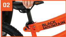
Open the guick-release seat clamp and unwind the hand-nut a couple of turns to fully release the clamp.
