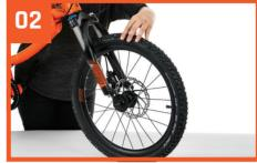
Insert the wheel bolts\* (you'll find them in the VIP box) either side of the wheel and leave enough space for the wheel to slot into the forks. For disc brakes, see the additional step 01A on the next page.
