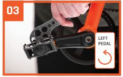
Once you have threaded them on fully by hand, finally tighten them up to 25Nm (18.4ft-lb) torque with the supplied 15mm spanner.
