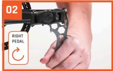
Make sure that you have the correct pedal for each side of the bike. On the end of each pedal axle you will find either a letter R (right) or a letter L (left).
