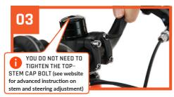
Replace the face plate, insert face-plate bolts and then evenly tighten each of them (not fully, just enough to hold the handlebars in place), making sure that the handlebars are in the correct position.
