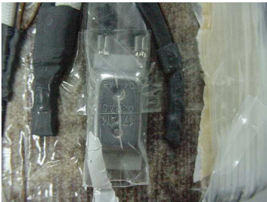
Thermal Link of Mains Transformer in Amplifier Module
