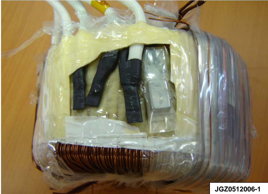
Location of thermal cut-out inside mains transformer (for ABM 500 series)
