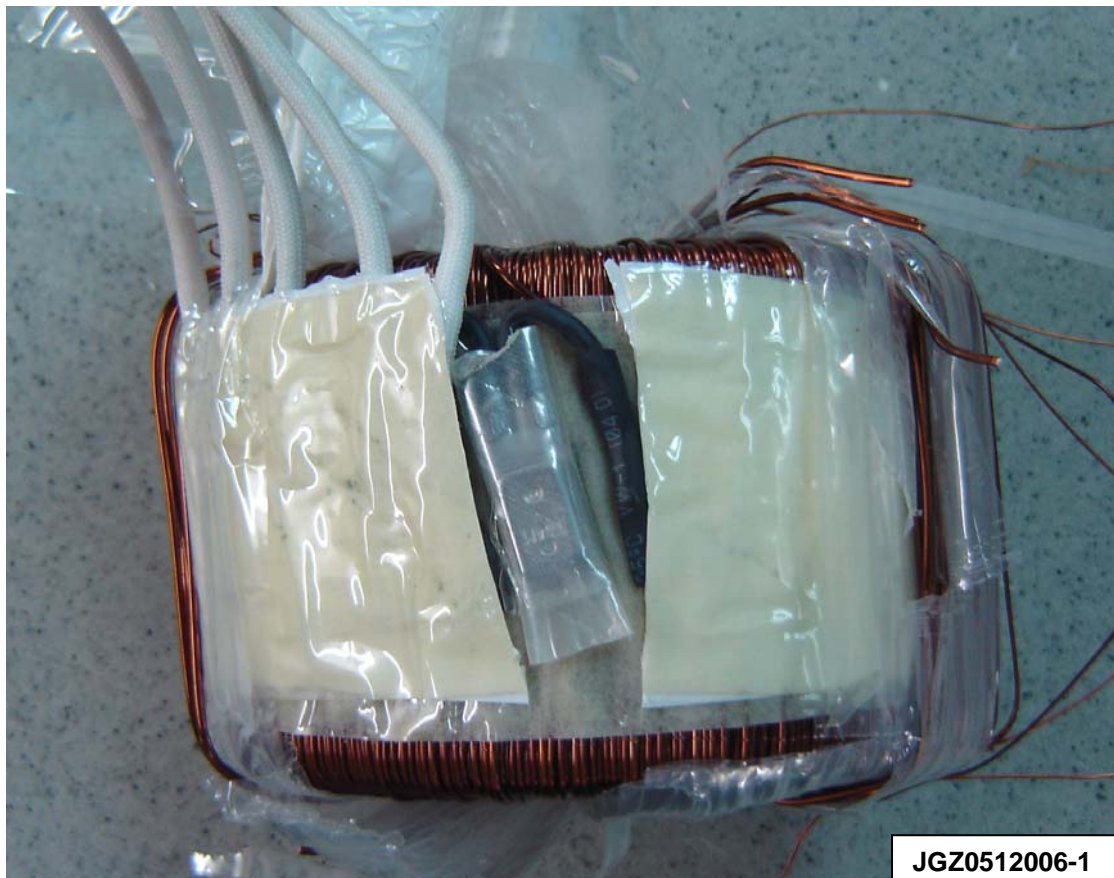
Location of thermal cut-out inside mains transformer for ABM 300 series
