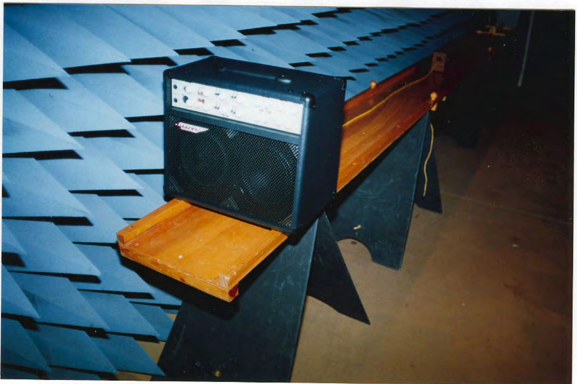
Photograph 14. Radiated Emissions: Disturbance power measurements – Typical Test Setup
