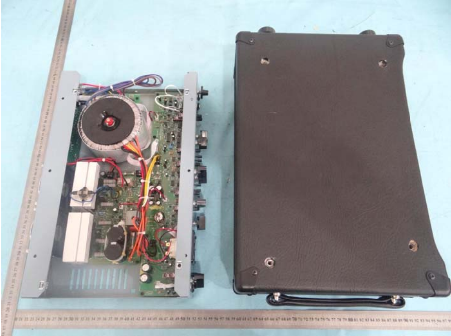
Figure 5 General Internal of the E.U.T.
