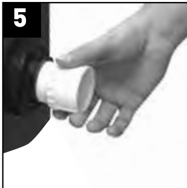
5 Attach a threaded male pipe adapter to lower bulkhead.
