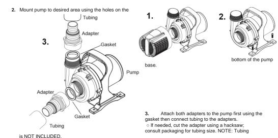
To prevent air from being taken in, ensure that unit and supply hose are always below the water level.
