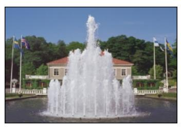
The Geyser nozzle is a water and air entraining venturi type, which augments the effect by adding water volume from the pool and aerating the mass. This method provides a heavy punch with moderate aeration to increase visibility. Compared to the Cascade nozzle, visibility is greater because the entrained air gives a roiling, white water appearance. Geyser nozzles are widely used in architectural fountains due to their high visibility and good wind resistance. Moderately "hard" in both
