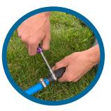
Layout the self-weighted airline in a line connected to the diffuser(s). Ensure a secure connection. You should not be able to twist the tubing on the fitting
