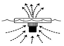
During unit operation, water is circulated from  $360^{\circ}$  around the unit as well as from below. Top intake for shallow water operation.
