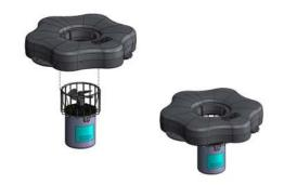
The motor unit attaches to the float using stainless steel hardware for a secure assembly. The single section, U.V. resistant, high density thermoplastic float, with closed cell foam filling allows for excellent durability with an attractive shape and low visibility.
