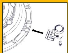
Snap-on clips included with RGB, Composite LED, and Stainless Steel LED systems.
