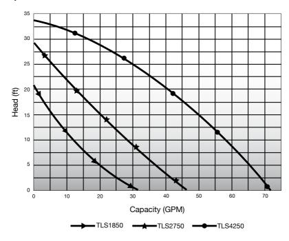
Discharge 1<sup>1</sup>/<sub>4</sub>" fpt • Elbow 1<sup>1</sup>/<sub>2</sub>" fpt Voltage 115v, 60 hz • Power Cord 20<sup>1</sup>
