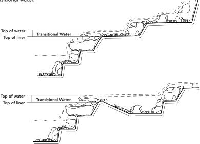
Below is an example of improper streambed construction. Stone, gravel and foam can be combined to make a barrier and create a waterfall, but that barrier will never be watertight. When the pump is turned off, the water will always drain down to the highest point of the liner. Improper construction greatly increases the water in transition.
