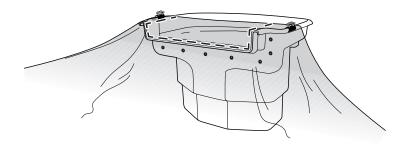
Remove the spring clips and pull the liner away from the face of the enclosure. Make sure that the front of the FilterFalls and the back side of the liner are clean and free of debris. Apply a consistent bead of Atlantic fish-safe silicone to the face of the FilterFalls along the center line of the threaded inserts.
