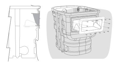
Use your fingers to hold the flange nut and a hand held screwdriver to tighten the screws. The serrations on the flange nut will grab the plastic enclosure once it makes contact, eliminating the need to use a wrench. Use caution when tightening the screws. The screws need only be snug for the silicone to make a seal.
