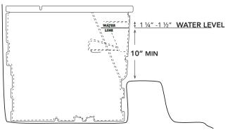
Place the Skimmer enclosure into the excavated hole. Check the top of the enclosure to make sure that it is level front-to-back and side-to-side. Check where your pre-determined water level falls on the face of the Skimmer enclosure. The water level needs to be between 1¼" and 1½" below the top of the weir door opening and even with the water level indicator molded on the side of the Skimmer. (PS15000 only)
