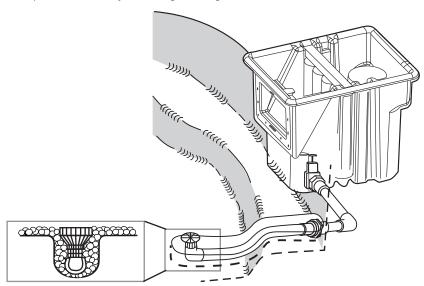
Drill-points have been provided on all compatible Skimmer models to show the proper location for the bulkhead fitting. See Figure 17. Drill the hole with a 3" hole saw and install the bulkhead following the bulkhead installation instructions on page 9.
