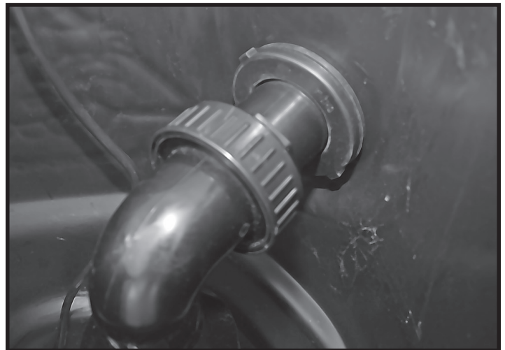
Ex. 15 One adaptor threads directly into the pump and the other threads directly into the bulkhead on the back of the skimmer. Apply silicone or Teflon tape (not included) to the threads of the fitting.
