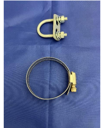
Example of U-bolt and hose clamp.
