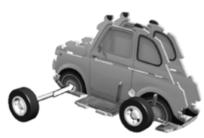
Insert the axis from step 6 into the front of the car.
