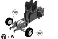
Attach rear wheels W onto the metal pieces from motor X.
