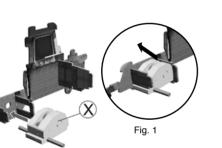
**6** + X Attach motor X by sliding it between pieces A4 and A5. See Fig. 1. Make sure the metal end pokes through the hole in piece A1.
