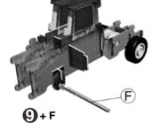
Slide metal axle rod F into the holes created by pieces B6.
