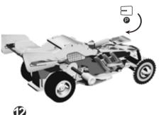
Attach the final piece, held horizontally, into the front of the car. This inserts above piece O. (see fig. 1 & 2).
