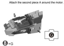
Attach motor X by pushing the metal piece
