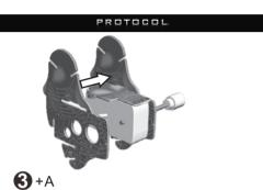
Attach secondary piece A to frame of the motor.
