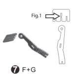
Attach piece G the middle slot of piece F (Fig.1) so that it is able to rotate freely.
