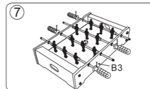
7. Insert the four small screws (parts B3) into the pre-drilled holes on the handles (parts A2) and athlete bars (parts T1, T2, T3, and T4) and tighten with the included screwdriver (part C1). Please use image 7 as a guide.
