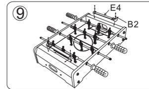
9. Install the two markers (parts E4) on the top of each short board (parts E1). Make sure to line up the pre-drilled holes on the markers and shortboards. Insert four screws (parts B2) into the pre-drilled holes and tighten using the included screwdriver (part C1). Please use image 9 as a guide.
