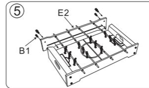
5. Slide the second long board (part E2) over the athlete bars (parts T1, T2, T3, and T4). Make sure the groove of the long board faces inward. Connect using 4 screws (parts B1). Please use image 5 as a guide.
