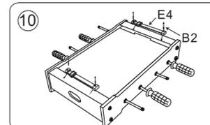
10. Turn the entire unit over to reveal the hockey side. Install the two markers (parts E4) on the top of each short board (parts E1). Make sure to line up the pre-drilled holes on the markers and shortboards. Insert four screws (parts B2) into the pre-drilled holes and tighten using the included screwdriver (part C1). Please use image 10 as a guide.
