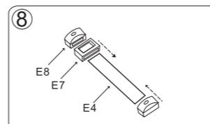
8. Slide the scoremarker (part E7) over the scorekeeper (part E4) and fix the scorecaps (parts E8) to each end. Please use image 8 as a guide.
