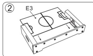
2. Insert the bottom board (part E3) into the assembled boards from step 1 following the grooves. Please use image 2 as a guide.
