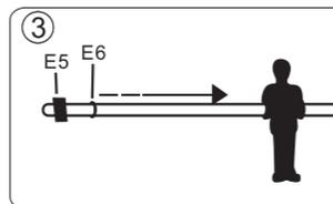
3. Slide one washer (parts E6) with the flat side towards the athlete on each end of the athlete bars (parts T1, T2, T3, and T4). Repeat this step using the rubber bumper (parts E5). Push the bumper and washer snug against each outside athlete. Please use image 3 as a guide.
