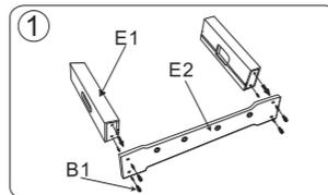
1. Assemble the two short boards (parts E1) with one long board (part E2) and connect using four screws (parts B1). Make sure the grooves on each board face inward. Please use image 1 as a guide.
