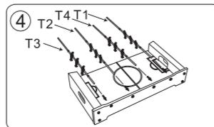
4. Install the four athlete bars (parts T1, T2, T3, and T4) into the holes of the long board (part E2). Make sure to alternate teams. Please use image 4 as a guide.
