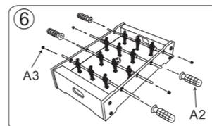
6. Slide on the four handles (parts A2) and the four covers (parts A3) over the athlete bars (parts T1, T2, T3, and T4) making sure everything fits tightly. The pre-drilled holes on the handle must line up with the pre-drilled holes on the athlete bars. Please use image 6 as a guide.
