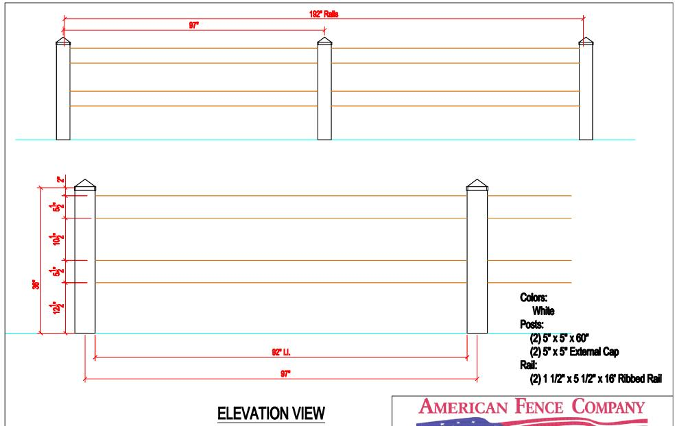
Picket spacing will vary 1/2"+/- based on panel widths. Installation will be full manufacture panels with partial panels on end to complete runs.
